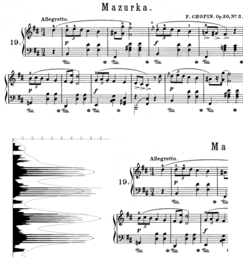
Figure 1. Top: first two systems from a scanned score. Bottom: horizontal projection and Gaussian smoothing of the top figure for locating systems in a page.
